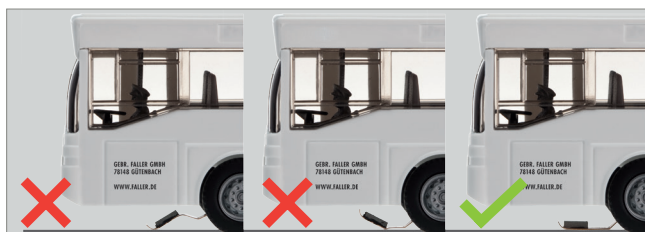
Fig. 3: Adjustment of the steering rod
