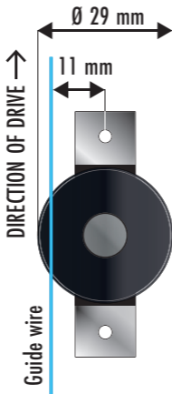
Fig. 9: Stop section with contact wire, Top view
