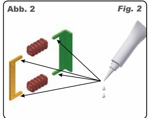
2. Glue the fuse (brass part) and the green support bracket to the isolators with a small amount of glue.
