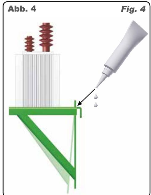
3. Assemble the electrical switch and fasten it with some glue.
