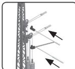
*Put the brackets into the fixingholes of the mast.*
