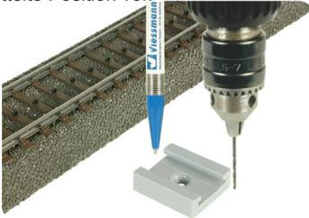
3. Mark the position of the screw with a pencil. Then remove the groundsocket and prick or drill the determined position with a ca. Ø1 mm drill.
