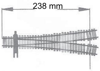
Note: To make a proper track approach to the deck, we recommend using a Walthers Code 83 #4 Wye turnout (948-8807) cut to the length of 238mm measuring from the single-track end, as shown in the diagram. It will be helpful to file a slight bevel on the inner edges of each rail head at the two-track end to guide wheels as they cross the gap.
