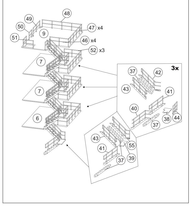
10) Glue left floor railings (46), right railings (52) and end railings (47) on floors (6, 7) and roof (9). Add railings (48, 49, 50 & 51) to roof as shown.
