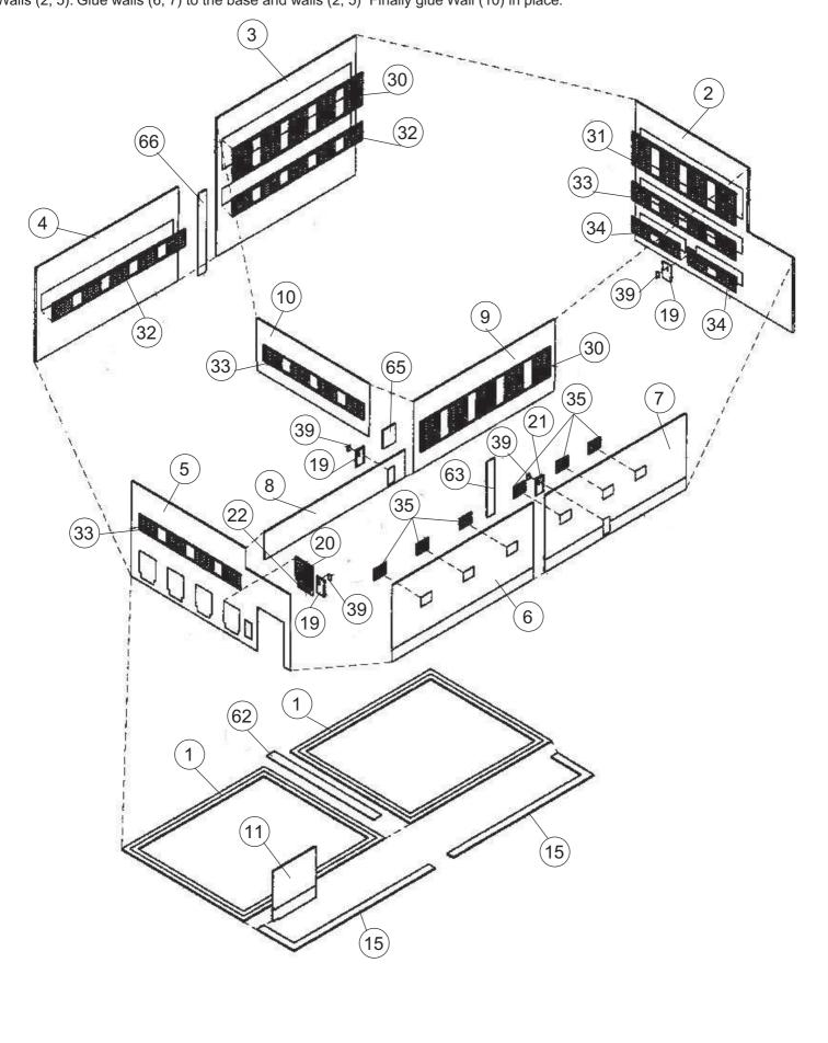
Glue Roofs (13) together end to end and reinforce the bottom with piece (64). Next, glue this assembly in place. Before gluing the other roofs (12), open up holes from the bottom of the roof pieces wherever a Small Stack (50) or Stack Vent Combo is desired. For Vents use Part 50 with Part 51 glued on top. For larger Vents glue part 52 and 53 together. Glue both Air Conditioner Units (54, 55, 56, 57) together and glue one to each Roof (12). For Small Stacks use Part 50.
