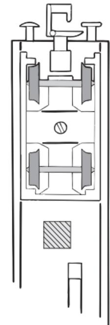
In order to ensure a troublefree switching function, the magnet is best positioned under the wagon chassis, near to an axle, or similary one of the bogies.
